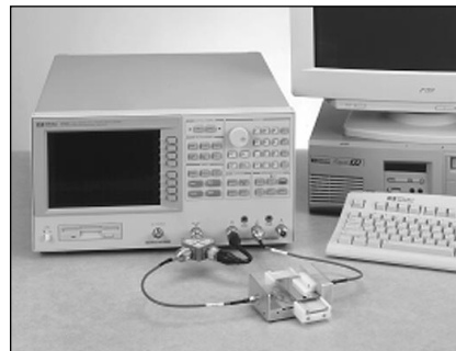
Permeance measurement system configuration with Agilent 4395A
